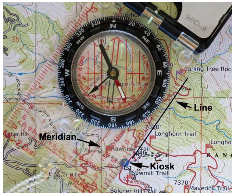
Figure 11: Setting a line with the bearing 035^\circ from the kiosk at the west parking lot of White Ranch Park.
