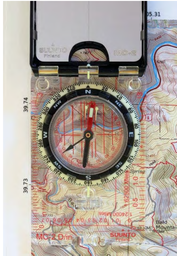
Figure 17: Orienting the map. The magnetic needle is aligned with the orienting arrow, which has the declination correction dialed in. The edge of the base is consequently lined up with true north.
