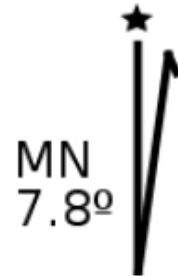
Figure 13: Magnetic declination diagram on a CalTopo map. The line with the star stands for true north; the half arrow stands for magnetic north.
