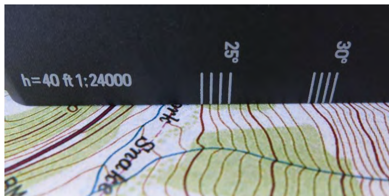
Figure 3 Measuring the slope of an area with scales on the MC-2 compass. The lower part of this avalanche chute has a slope of 25^\circ .
